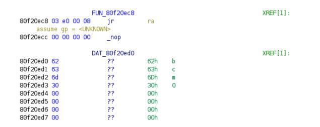
Given that the **.data** segment is at the end of the firmware file, it ends with a large amount of null bytes.
